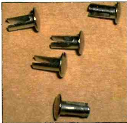
Photo F. I found these split rivets at my local small-town ACE Hardware store. Someday I'll replace them with the proper and more authentic looking hollow brass rivets, when a source is found.
